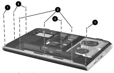
Removing the Top Cover Screws
